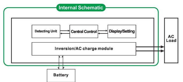
1.1 Normal working mode (ON): No matter it's connected AC loads or not the inverter always convert DC to AC. The LCD of the inverter displays the output voltage. The power consumption in normal working mode is a little higher than in sleep mode
