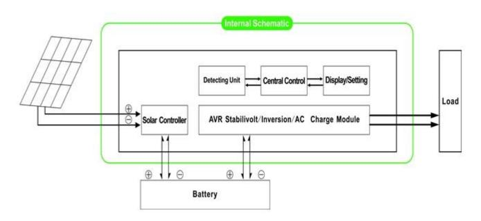
1.1 Normal working mode FREQUENCY in the LCD display is set to 01. No matter it's connected AC loads or not, theinverter always convert DC to AC. It'sready to supply power to the AC loads. In this mode, the LCD will displayoutput voltage as bellow:
