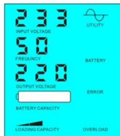
Battery unavailable, utility supply power
