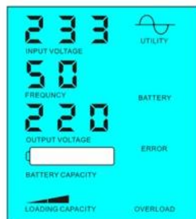
Battery unavailable, utility supply power
