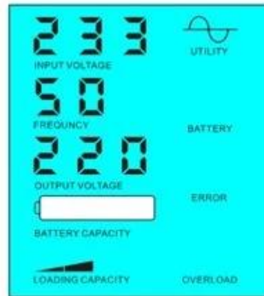
Battery dead, utility supply power
