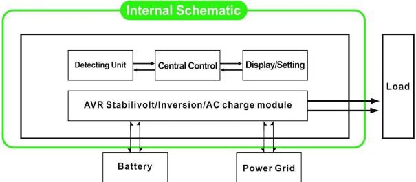
2.1 Utility first (AC first) battery standby mode: FREQUENCY in the LCD display is set to 01. When utility and battery are connected to the inverter, utility will supply power to the loads prior. When utility is cut off, the battery will automatically continue to supply power via power inverter.
