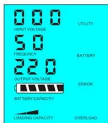
Load's power > 5% of inverter's rated power
