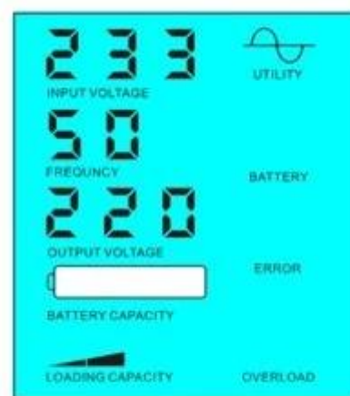
Battery dead, utility supply power
