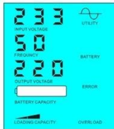
Battery dead, utility supply power
