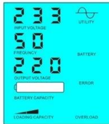
Battery dead, utility supply power
