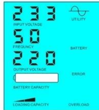
Battery dead, utility supply power
