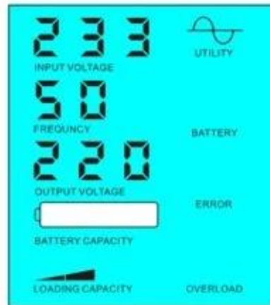
Battery dead, utility supply power
