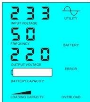
Battery dead, utility supply power
