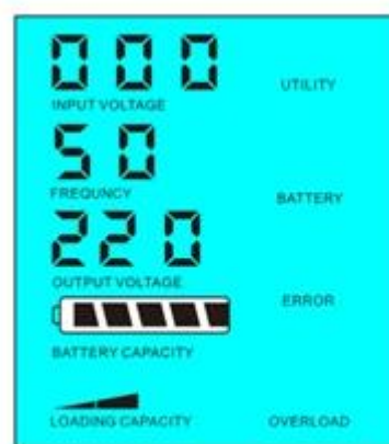
Load's power > 5% of inverter's rated power
