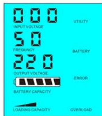
Load's power > 5% of inverter's rated power
