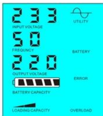
Utility supply power and charge battery
