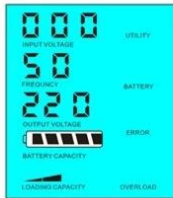
Load's power > 5% of inverter's rated power
