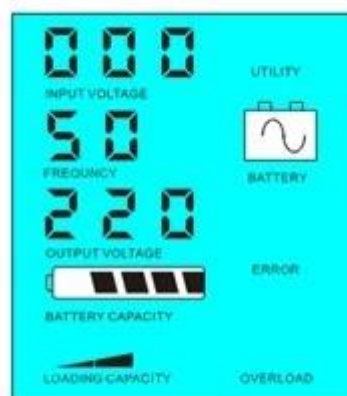
Without utility and battery supply power
