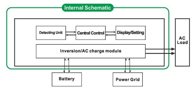
3.1. Utility first battery standby UPS mode (on the panel turn the button to "AC") When utility and battery are connected to the inverter, utility will supply power to the loads prior. When utility is cut off, the battery will automatically continue to supply power via power inverter. Steps are as below:
