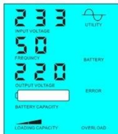
Battery dead, utility supply power
