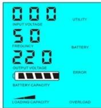
Load's power > 5% of inverter's rated power
