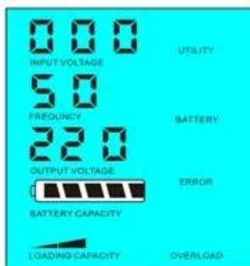
Load's power > 5% of inverter's rated power
