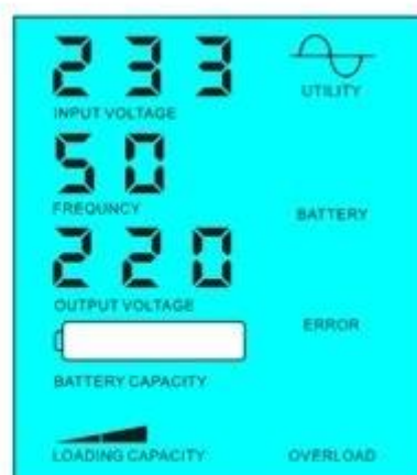
Battery dead, utility supply power
