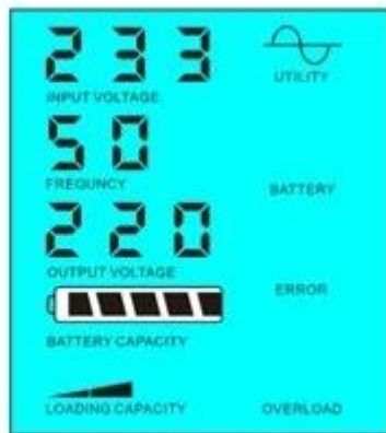
Utility supply power and charge battery
