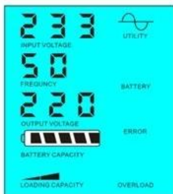
Utility supply power and charge battery
