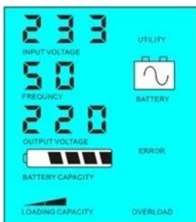
Battery has power
