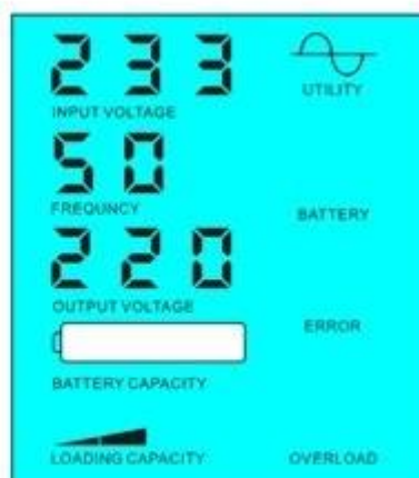
Battery dead, utility supply power
