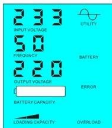
Battery dead, utility supply power
