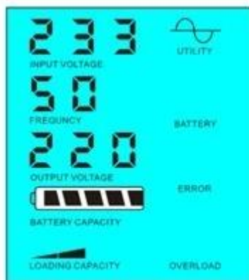
Utility supply power and charge battery
