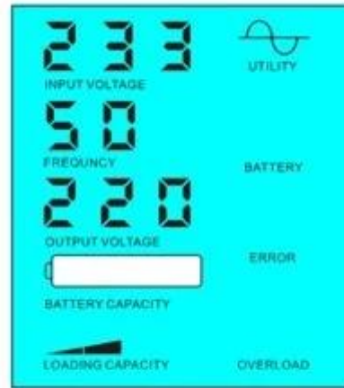
Battery dead, utility supply power
