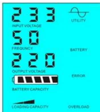
Utility supply power and charge battery
