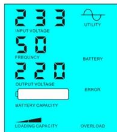
Battery unavailable, utility supply power
