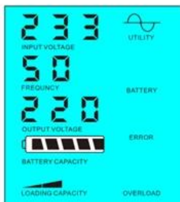
Utility supply power and charge battery
