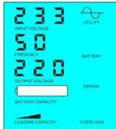
Battery dead, utility supply power
