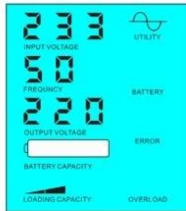
Battery dead, utility supply power
