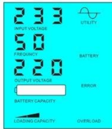
Battery dead, utility supply power
