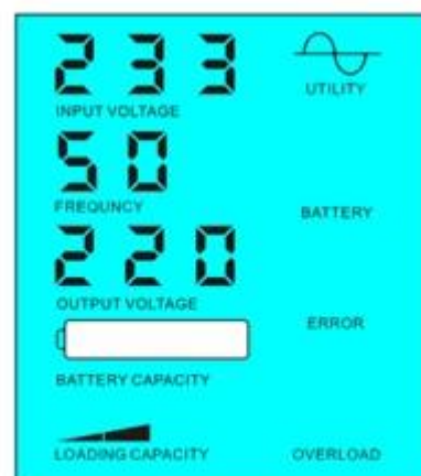
Battery unavailable, utility supply power
