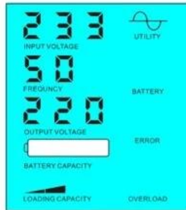
Battery dead, utility supply power
