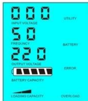
Load's power > 5% of inverter's rated power
