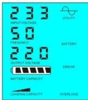
Utility supply power and charge battery
