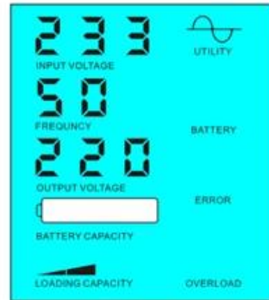
Battery unavailable, utility supply power
