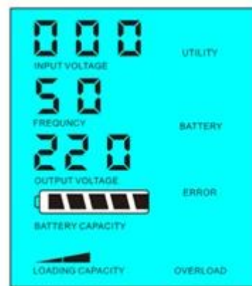
Load's power > 5% of inverter's rated power
