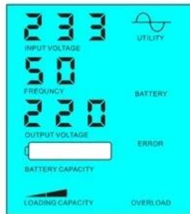
Battery dead, utility supply power
