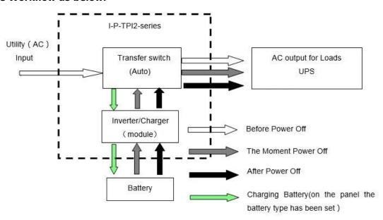
3.2. Battery first utility standby UPS mode (on the panel turn the button to "DC").
