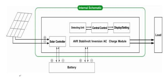
1.1 Normal workingmode []FREQUENCY in the LCD display is set to01. No matter it's connected AC loads or not, the inverter always convert DC to AC.
