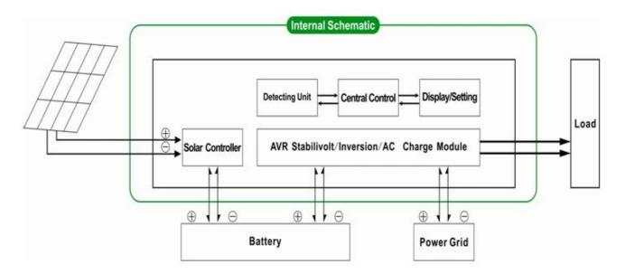
2. UPSfunction When the inverter is connected to battery and utility, users can set it to utility first (AC first) batterystandby mode or battery first (DC first)utility standby mode.
