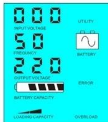
Without utility and battery supply power
