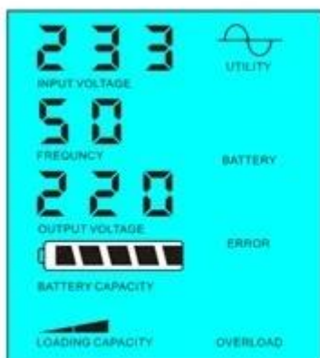
Utility supply power and charge battery
