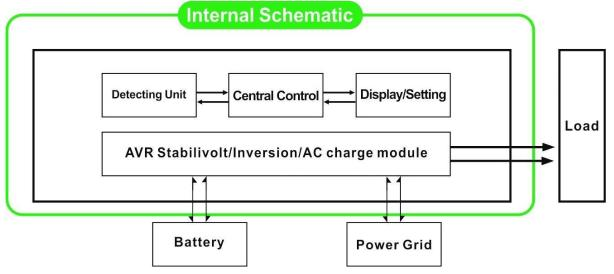
2.1 Utility first (AC first) battery standby mode: FREQUENCY in the LCD display is set to 01. When utility and battery are connected to the inverter, utility will supply power to the loads prior. When utility is cut off, the battery will automatically continue to supply power via power inverter.
