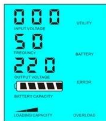
Load's power > 5% of inverter's rated power
