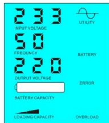
Battery unavailable, utility supply power
