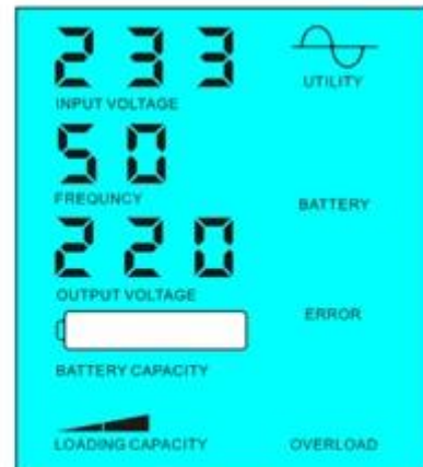
Battery unavailable, utility supply power
