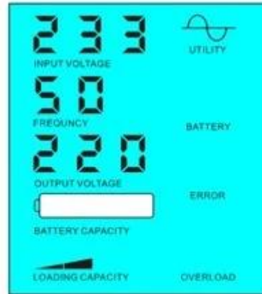
Battery dead, utility supply power
