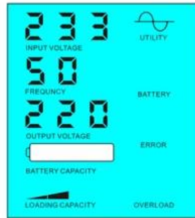
Battery unavailable, utility supply power
