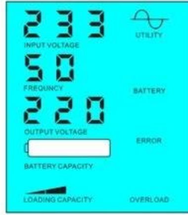
Battery dead, utility supply power
