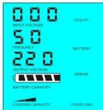
Load's power > 5% of inverter's rated power
