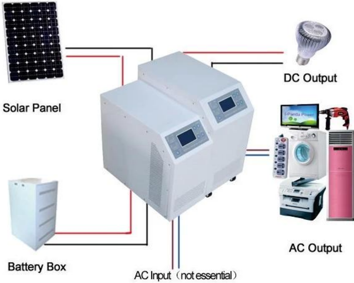
I-P-HPC-Series Inverter+Solar Controller
