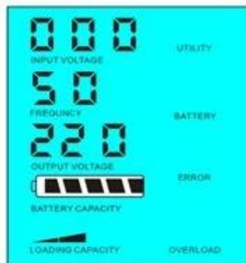
Load's power > 5% of inverter's rated power
